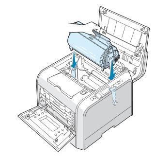
**CAUTION**: Insert the imaging unit carefully so as not to scratch and damage the surface of the green roller.
